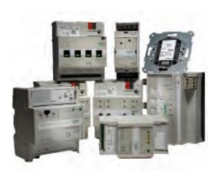
Due to Link-Power-technology, both data and the supply voltage for the control electronics can be transmitted via the LON network. Particularly, if the I/O modules are applied peripherally the complexity of cabling is minimised. LPT devices can be operated in combination with FTT devices in one subnet, but then they require an extra LON Power Supply
